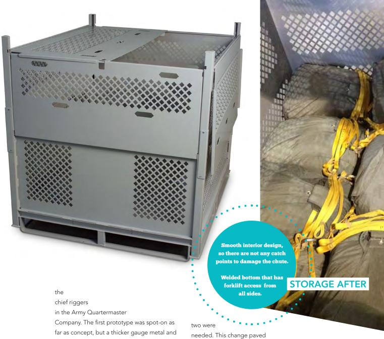
Company. The first prototype was spot-on as far as concept, but a thicker gauge metal and a larger size was needed. The next iteration addressed and solved the durability issue by adding diamond perforated 12 ga. steel panels for visibility and ventilation and an 11 ga. steel frame for strength and rigidity. Protected
