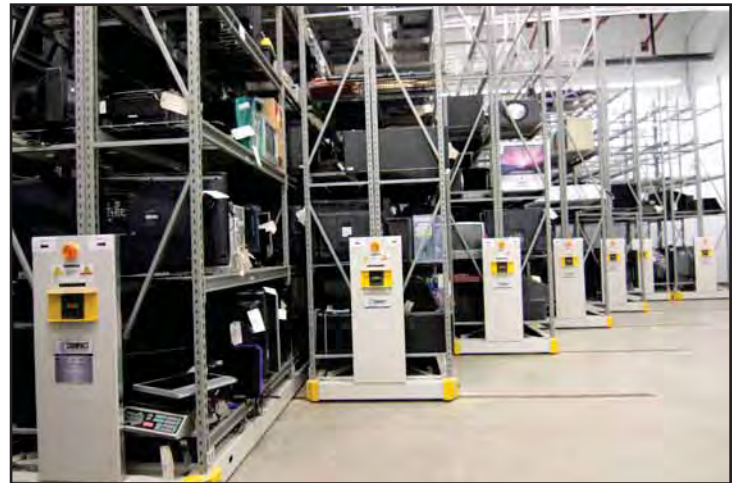
Staggered or tiered carriages maximize storage space when angled walls are present.
