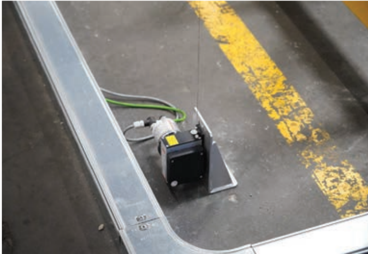
Wire encoder for maximum precision
