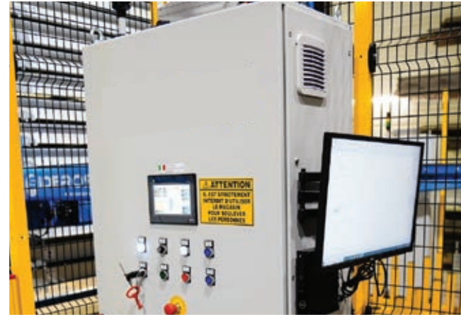
HMI touch screen and 21" screen for warehouse WMS software
